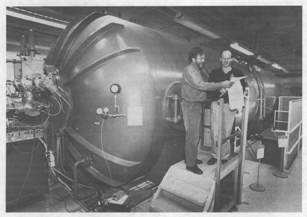
BIG MACHINE, SMALL BEAM — Dan Morse (left) and Mark Hildner (both 8347) examine test results at the Van de Graaff FN tandem accelerator located at Lawrence Livermore's multi-user tandem laboratory. The 10foot-diameter accelerator and a series of magnetic lenses produce a 2-micron proton beam that is being used by Sandia researchers to develop stronger, more durable materials for artificial heart valves.
